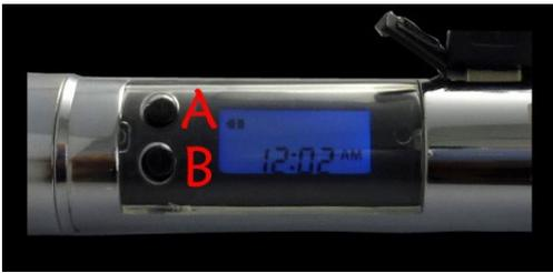
1. Press A button 3s to boot, showing the cumulative amount of smoking E-liquid, the remaining percentage of E-liquid and the remaining battery capacity. Press A button 3s to shutdown, showing the time;
