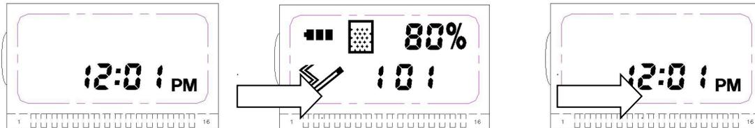
2. Every time smoking, E-liquid would be reduced, the cumulative number of smoking mouth will increase. When the E-liquid is content reduces to 0%, the lampblack symbol of E-liquid will have flash warning;
