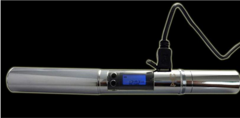
(2) Normal shutdown, rotate the battery cover, remove the lithium battery, then put the lithium battery inside the wall charger directly to charge. When the charger from the red light turns to green light, it means the battery is fully charged.
