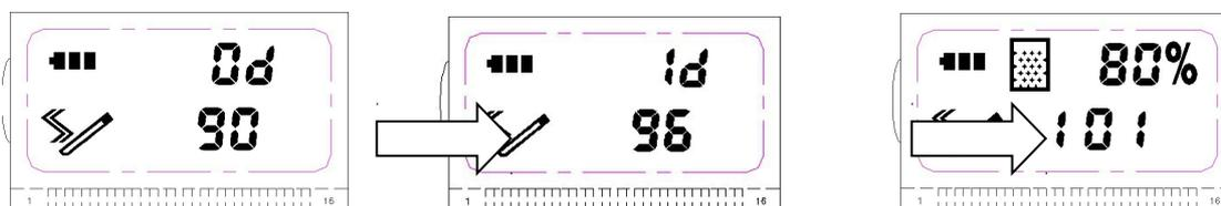
5. In the boot mode, press the B button and A button for 5S at the same time to clear the record of smoking history. "CLr" flashes 2 times back to next.
