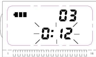
4. Set the hours. Press A button add 1, AM / PM setting automatically followed hour setting and switch;
