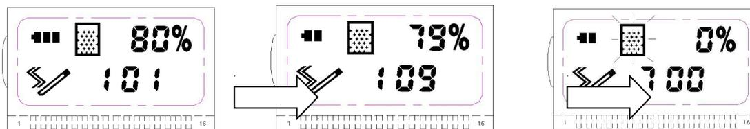
3. Battery symbol cell represents the number of battery power, when battery power is exhausted, the battery symbol will have flashing warning and stop smoking;
